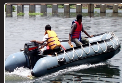
INFLATABLE RESCUE BOAT As per IRS approved design, with or without OBM
